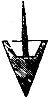
Fig. 14—Represents a section through the axis of a cast-iron shoe and wrought-iron bolt for a pile
